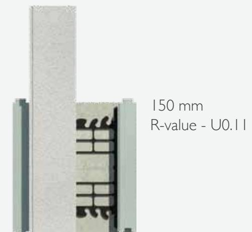
150 mm concrete core U-Value ratings based on exterior brick finish
